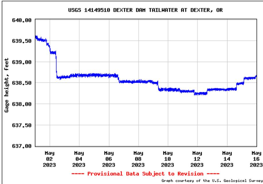
**Figure 50. Gauge Height (feet); below Dexter Dam, Middle Fork Willamette**
