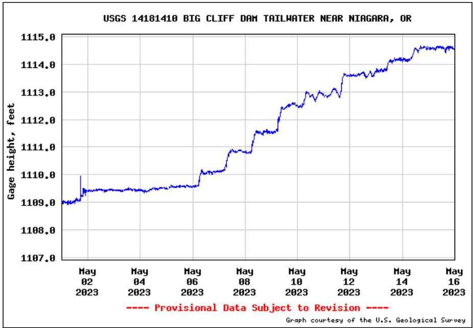
**Figure 14. Gauge height (ft); below Big Cliff Dam**
