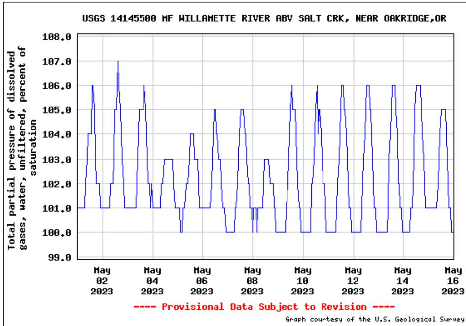
**Figure 68. Total Dissolved Gas Saturation (%); below Hills Creek Dam – Middle Fork Willamette River**
